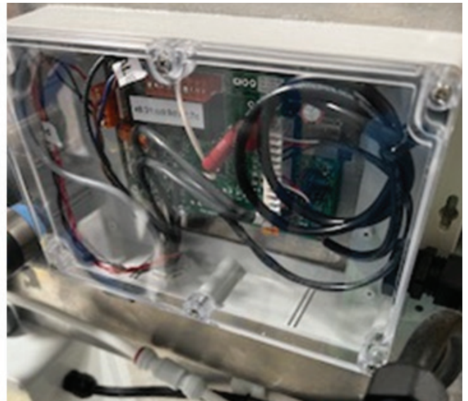
Location of float switch connection leads in front panel enclosure.
